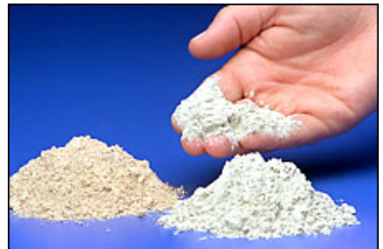
TURNING CO 2 TO MINERALS - Gaseous carbon dioxide can be captured and converted into these environmentally-safe, magnesite minerals. The brown mineral is produced when olivine is used in the reaction; the white powder is produced when serpentine is used.
