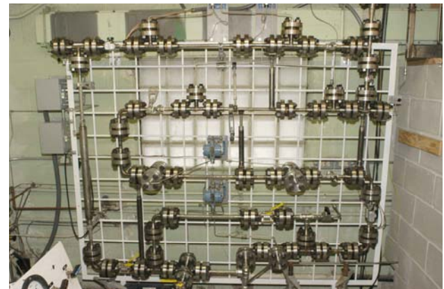
Figure 12. Laboratory-scale flow loop reactor.
