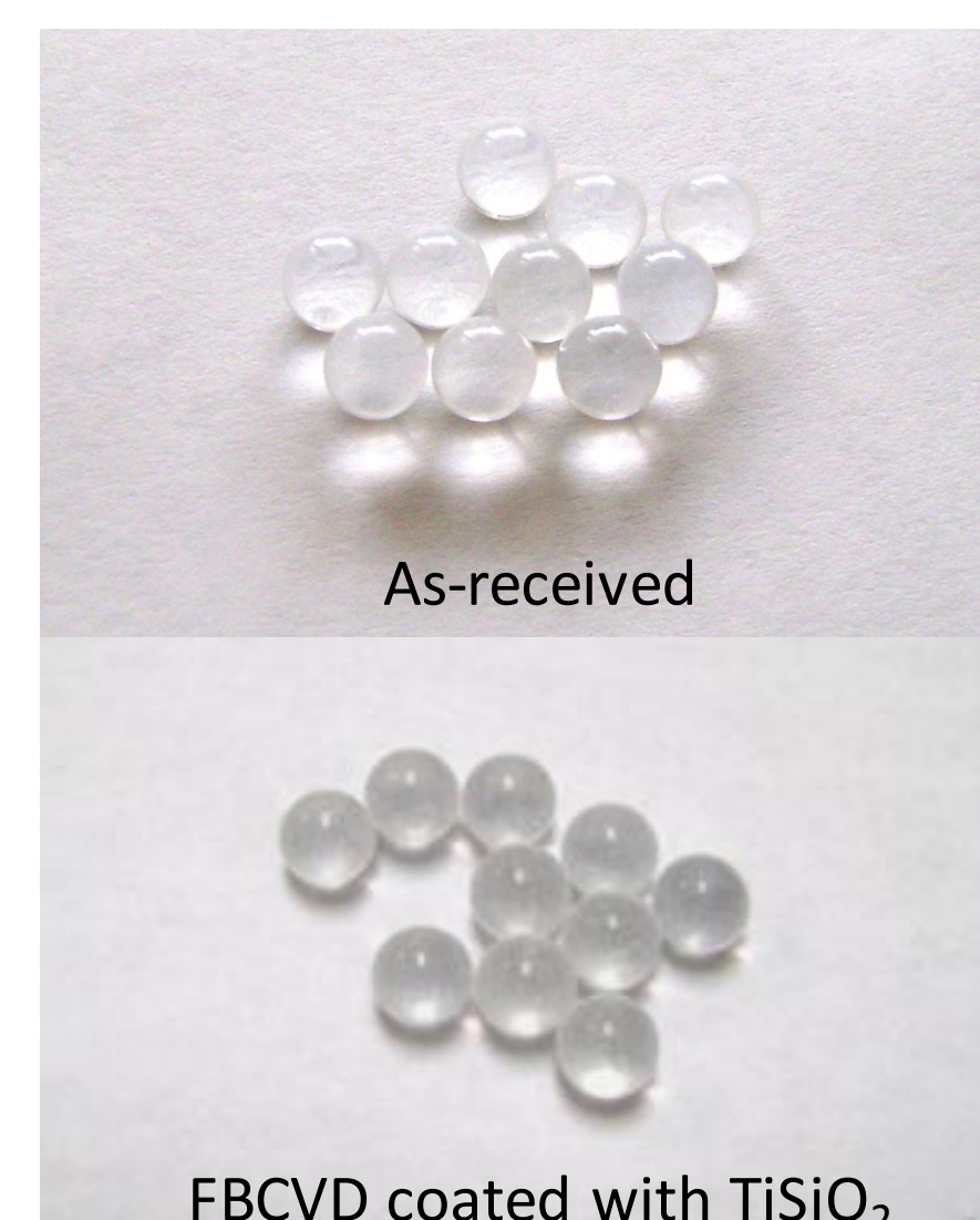
Figure 6: Borosilicate glass beads (6 mm diameter) with \text{TiSiO}_2 coating deposited by FBCVD at SMI.
