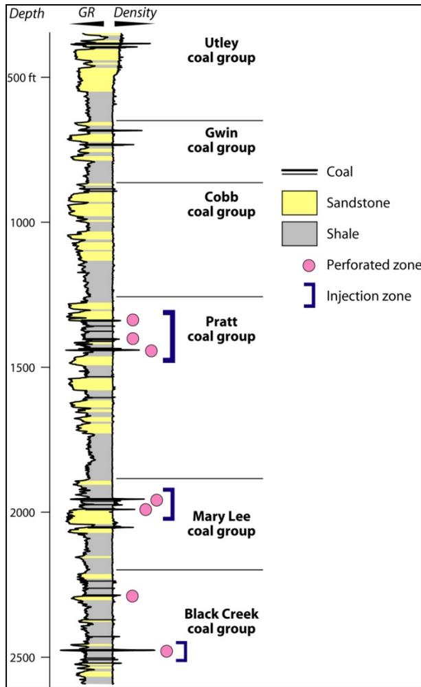
Figure 2. Well log showing stratigraphic section and injection zones in the test area
