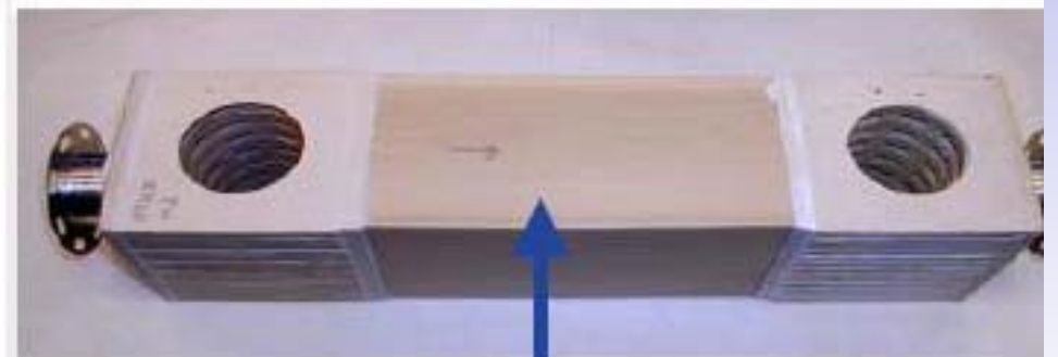
ASSEMBLED CERAMIC HEX MODULE FABRICATED BY HYDRO
