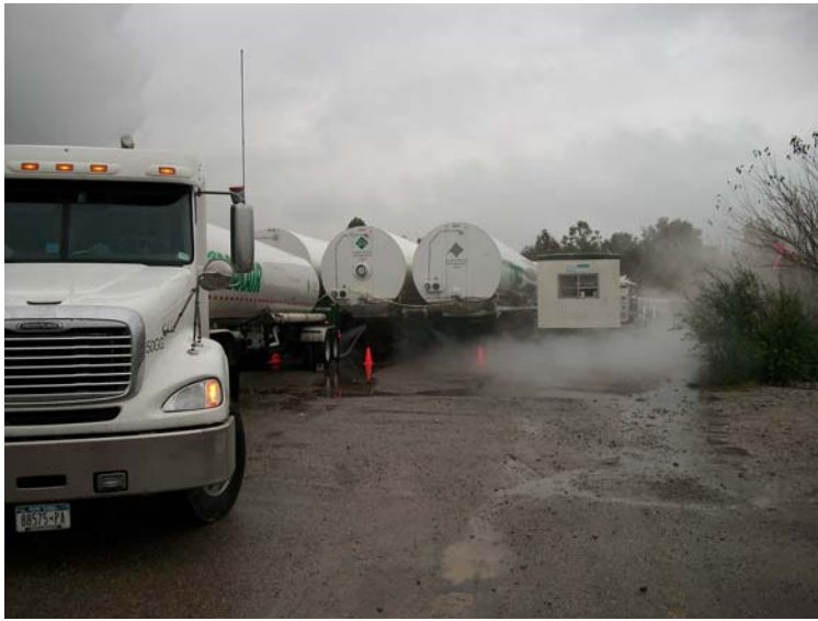
Figure 1. Left: A temporary supply of CO 2 was stored on site in storage tanks. The carbon dioxide that was used for this test was the same in composition as that routinely used in the food industry. It was transported as a liquid by standard delivery trucks. Right: The injection target (Mt. Simon Sandstone) is more than a half mile below ground. The injection well is shown in the center.
