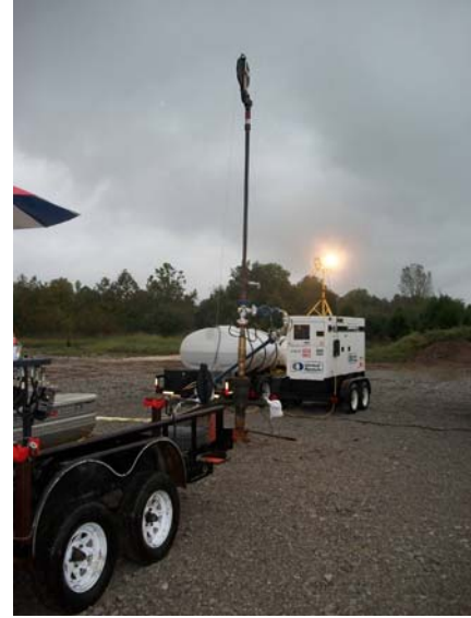
Figure 1. Left: A temporary supply of CO 2 was stored on site in storage tanks. The carbon dioxide that was used for this test was the same in composition as that routinely used in the food industry. It was transported as a liquid by standard delivery trucks. Right: The injection target (Mt. Simon Sandstone) is more than a half mile below ground. The injection well is shown in the center.
