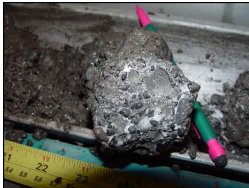
Photograph of a gas-hydrate-bearing sediment core from the Mallik 5L-38 Gas Hydrate Production Test Well. The white material in this photo is the gas hydrate. (Courtesy of the Mallik 2002 Gas Hydrate Production Test Well Program)
